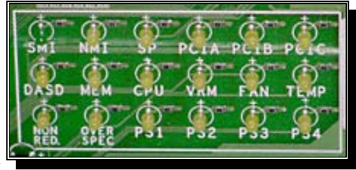
Figure 1. Light Path Diagnostics panel
